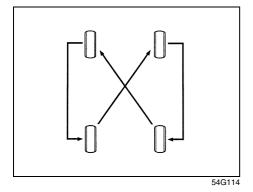
To avoid uneven wear of your tires and to prolong their life, rotate the tires as illustrated. Tires should be rotated as recommended in the periodic maintenance schedule. After rotation, adjust front and rear tire pressures to the specification listed on your vehicle's Tire and Loading Information Label.
